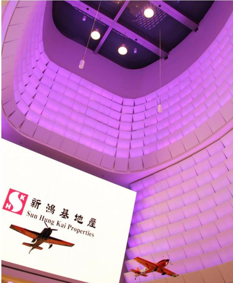
8 adjustable hanging points at the 2/F Atrium (each with 250kg safe working load) are attached to the steel wires powered by the winches at 6/F Skylight's equipment room (bottom right) to ensure safe lifting.
